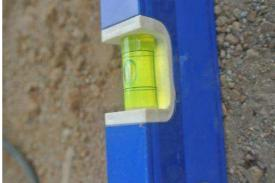
Sprit levels are used to determine whether a surface is correctly vertical or horizontal. A surface is correct when the bubble is between the two black lines.
